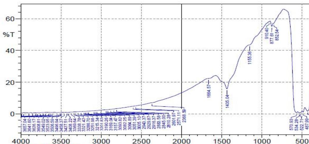
Figure (4): The FT-IR absorption spectrum of copper oxide.
