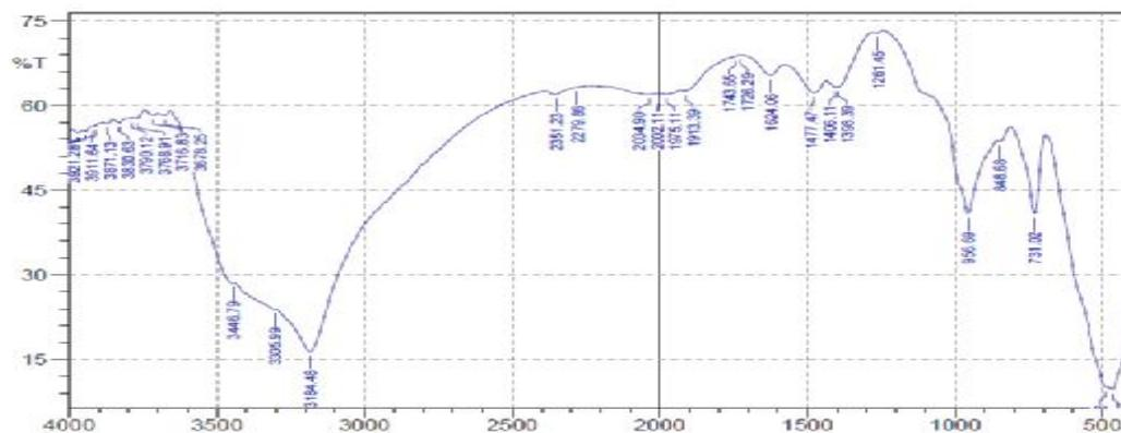
Figure (5): The FT-IR absorption spectrum of copper oxalate.
