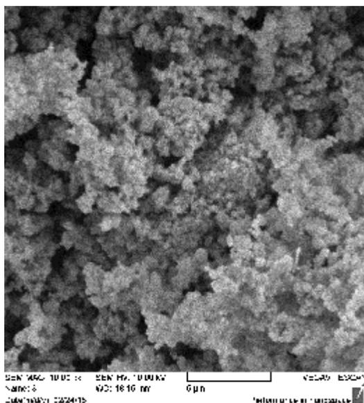
Figure (9): The scanning electron microscope image of copper oxide.
