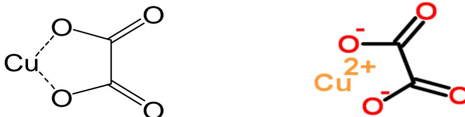
Figure (3): Copper oxalate formula, in which one molecule of copper cation attached to one oxalate anion.
