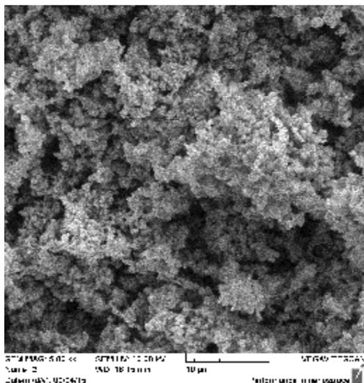
Figure (8): The Scanning Electron microscope image of copper oxalate.
