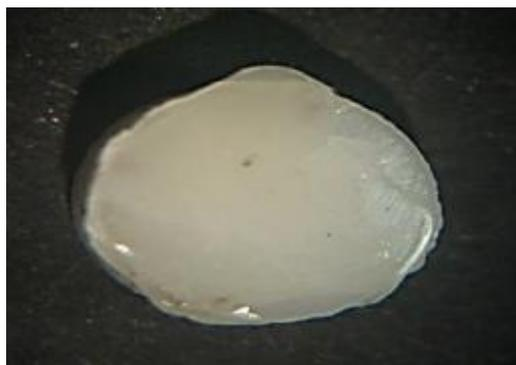
Figure(9): Mixed failure.
