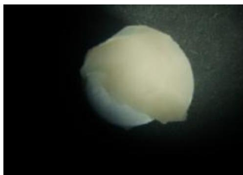
Figure(8): Cohesion failure of composite.
