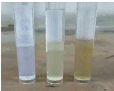
Figure (2): Synthesis of silver nanoparticles by supernatant of *E. coli*
