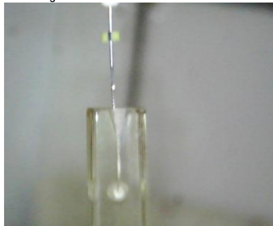
Figure (1): The k-file was applied at right angle to the surface of endo. block
