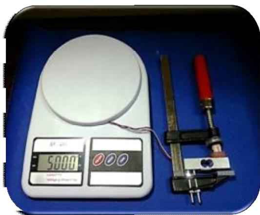
Figure (3): The sample scurried to the specimen holding device attached to a digital scalar
