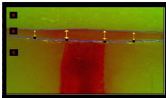
Figure(4): Digital image was captured and represented marginal gab measurement, A: Crown, B: Marginal gap, C: Master die
